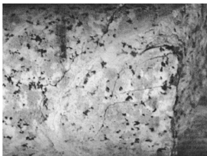
Fig. 5. Cracks due to laumontite crystallization.
