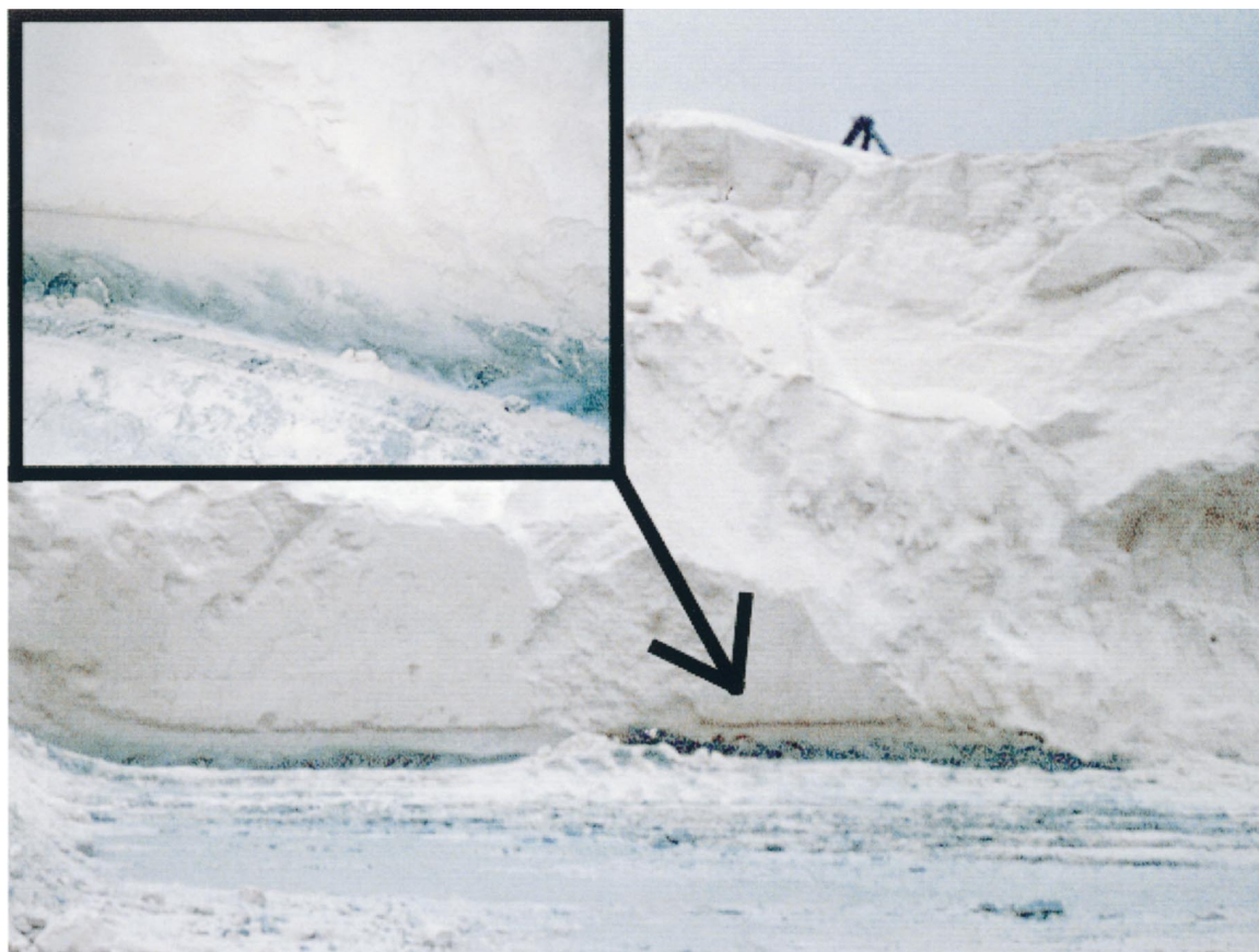
Fig. 8. Exposed face of slag stockpile showing the blue-green coloration at the base.
