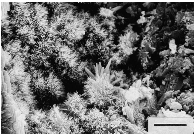
Fig. 5. Detail of the microstructure of CSH phases in the matrix of the nineteenth century hydraulic mortars (SMKC7). Scalebar=10 \mu\text{m} .
