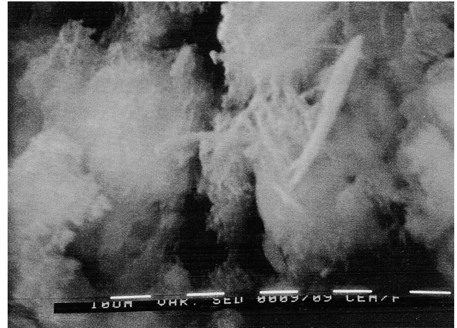
Fig. 2. Microstructure of the evaporation residue of water sample F (marker = 1 μm).
