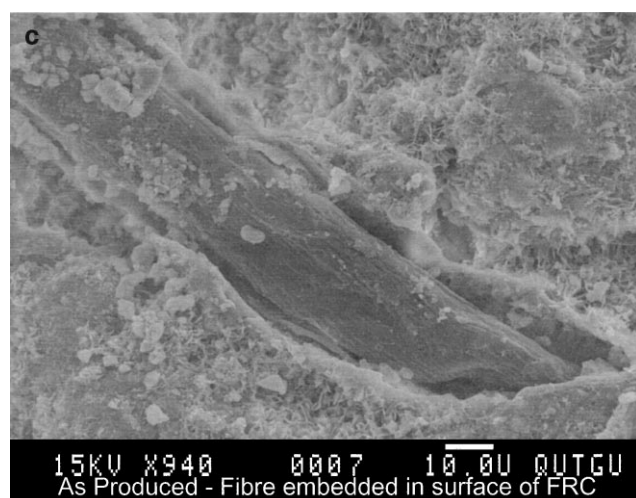
Fig. 5. Scanning electron micrographs of control samples of SRC and FRC.
