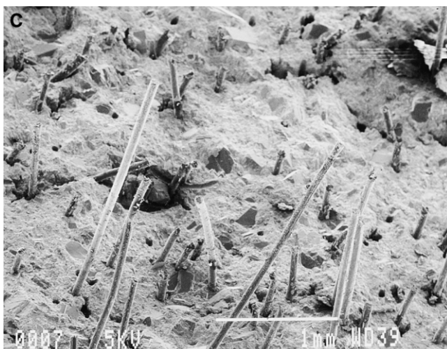
Fig. 8. Fracture surface of extruded fiberboard with different fibers. (A) PET fiberboard (Batch #3), (B) AR glass fiberboard (Batch #4), (C) PO fiberboard (Batch #5), and (D) PVA fiberboard (Batch #6).
