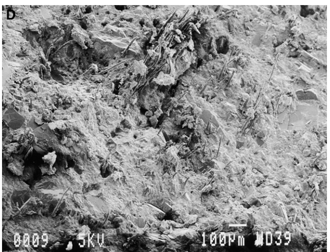
Fig. 8. Fracture surface of extruded fiberboard with different fibers. (A) PET fiberboard (Batch #3), (B) AR glass fiberboard (Batch #4), (C) PO fiberboard (Batch #5), and (D) PVA fiberboard (Batch #6).
