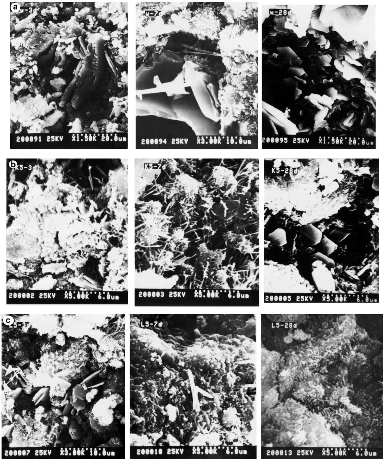
Fig. 4. SEM photos of hydrated samples. (a) The white Portland cement. (b) The white Portland cement with 5% admixture. (c) The white Portland cement with 5% K admixture.
