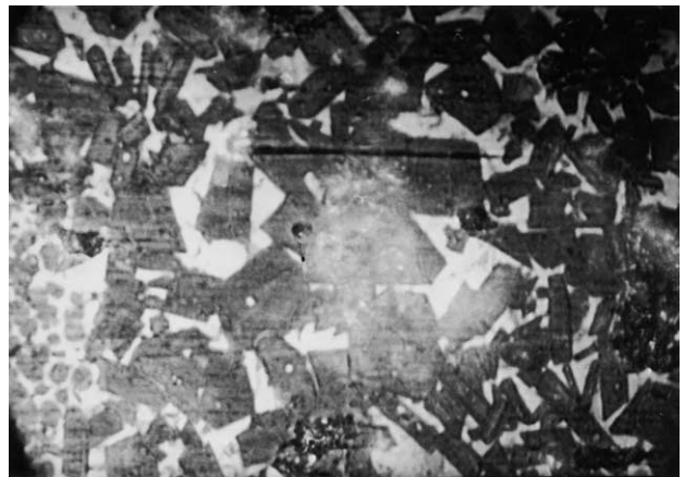
Fig. 3. Mineralogical distribution in clinker which was subjected to electric heating at 1200 °C and microwave heating for 60 s.
