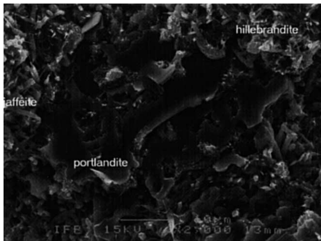
Fig. 8. SEM image of secondary electrons of the \text{C}_3\text{S} hydrated sample ( \text{W/C}=0.44 ) at 200^\circ\text{C} under 450 bars during 2 months ( \times 350 ).
