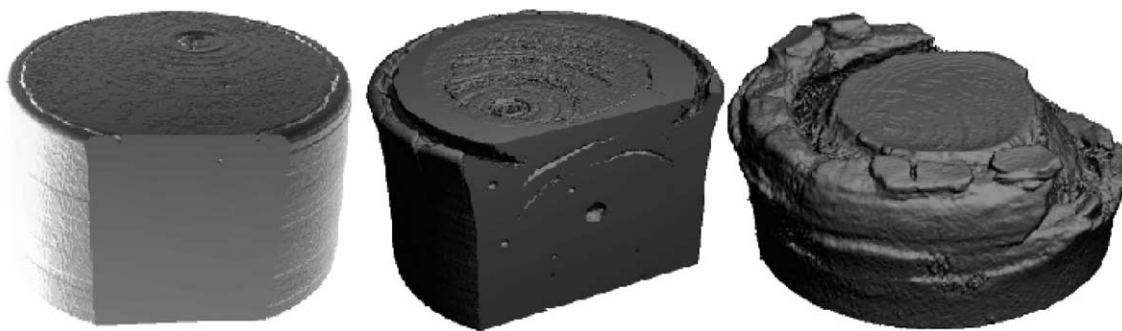
Fig. 2. Microtomography-based 3D renderings of damaged cement paste samples with damage levels 1 (w/c 0.45), 2 (w/c 0.50) and 3 (w/c 0.60), left to right, respectively.
