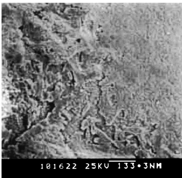
Fig. 2. SEM micrograph of fractured old concrete substrate using YJ-303 primer.
