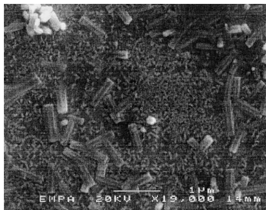
Fig. 21. SE micrograph of interstitial phase after 24 h hydration in extracted solution with 0.004% HP, prisms and rod-like deposits.
