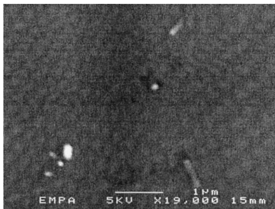
Fig. 19. SE micrograph of interstitial phase after 24 h hydration in extracted solution with 0.004% CP, prisms.
