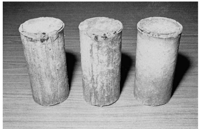
Fig. 4. OPC concrete cylinders exposed to magnesium sulfate solution for 12 months. Some expansion, cracking, and loss of concrete at the corners were observed.
