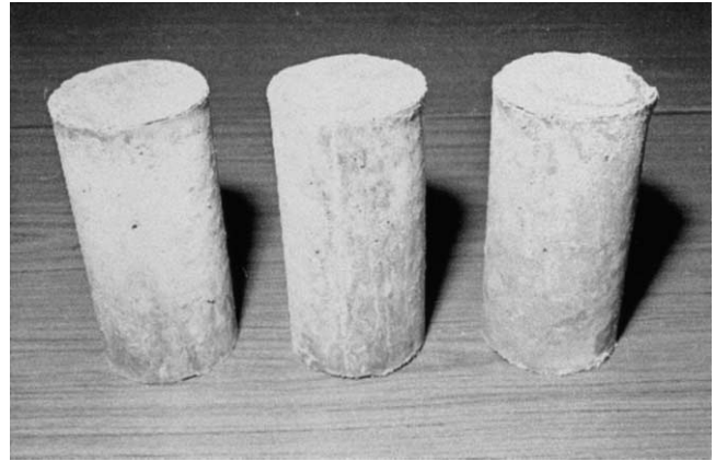
Fig. 3. OPC concrete cylinders exposed to sodium sulfate solution for 12 months. Some expansion and cracking on the surface of concrete specimens are evident.
