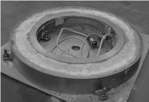
Fig. 3. ASG to evaluate the cracking susceptibility of mortars. Strain gauges are mounted on the inside of the inner steel ring to measure the deformation. During measurement, the top surface is covered with acrylic glass. The mortar ring has a cross-section of 50×50 mm [7].
