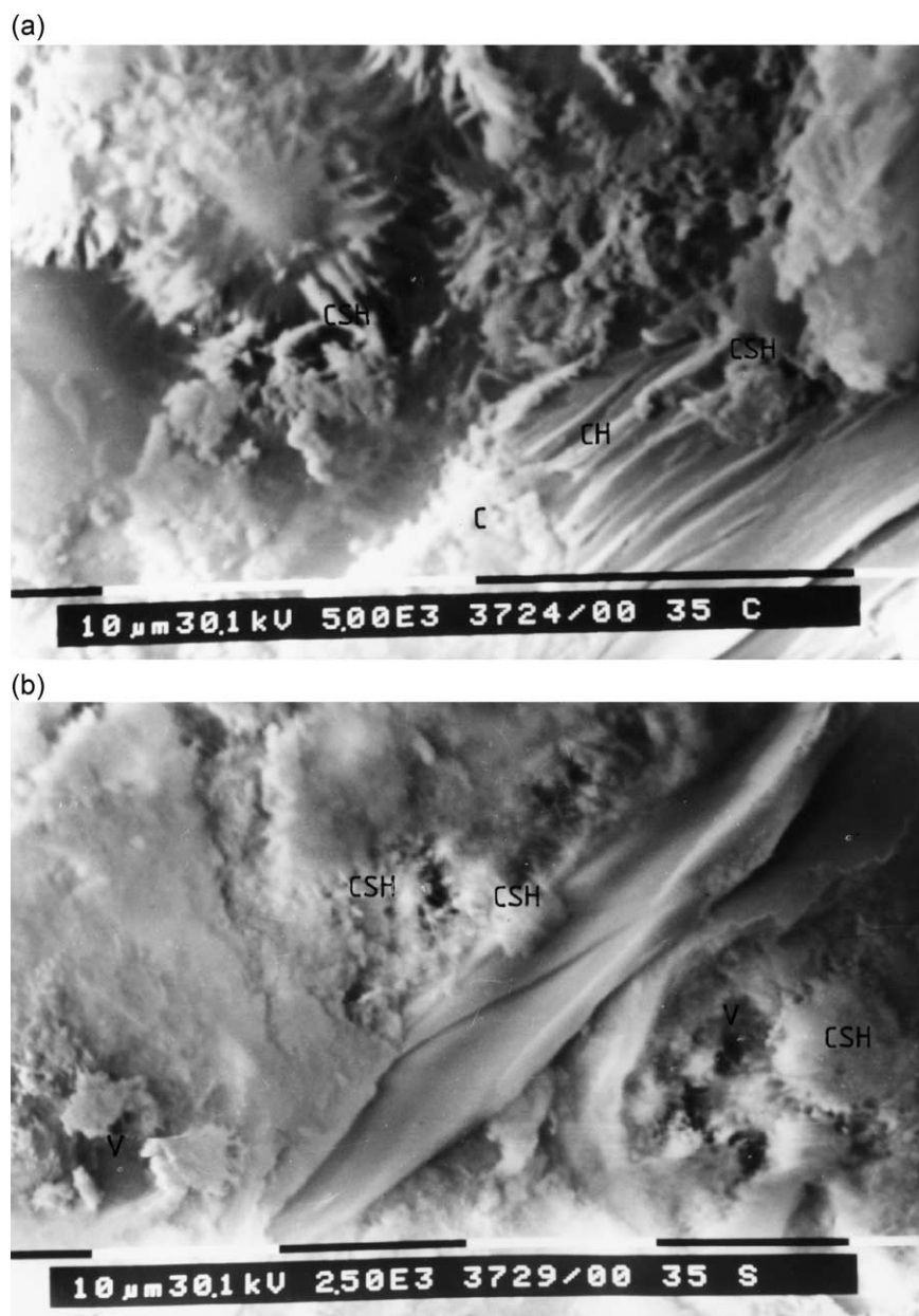
Fig. 6. SEM micrographs of hardened concrete at 300 °C: (a) core, (b) surface.
