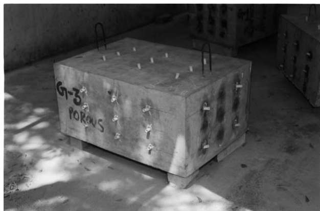
Fig. 6. Location of the grout ports fixed using aluminium pipes.
