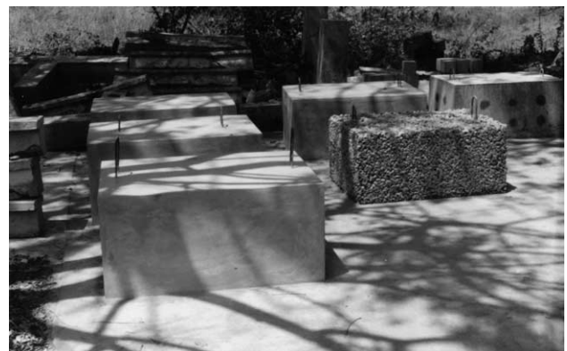
Fig. 4. No-fines concrete blocks before and after plastering.
