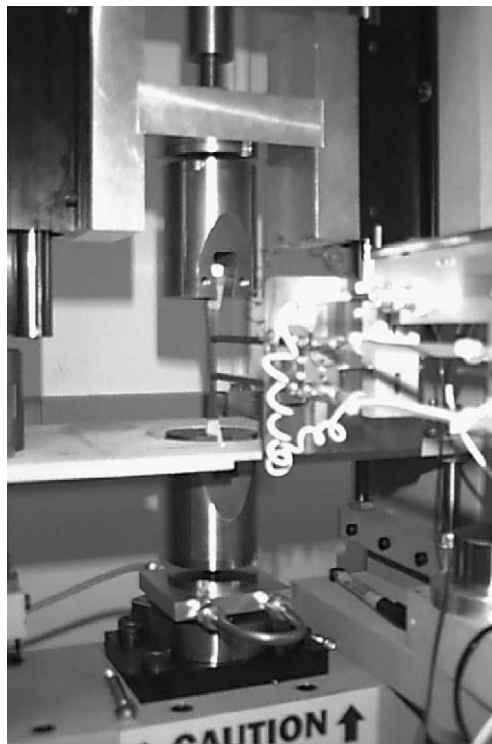
Fig. 5. Overview of the composite tensile testing deadweight creep frame.
