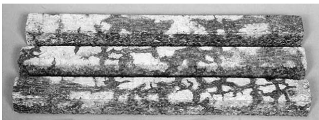
Fig. 3. Map cracks on the surface of the control specimens.
