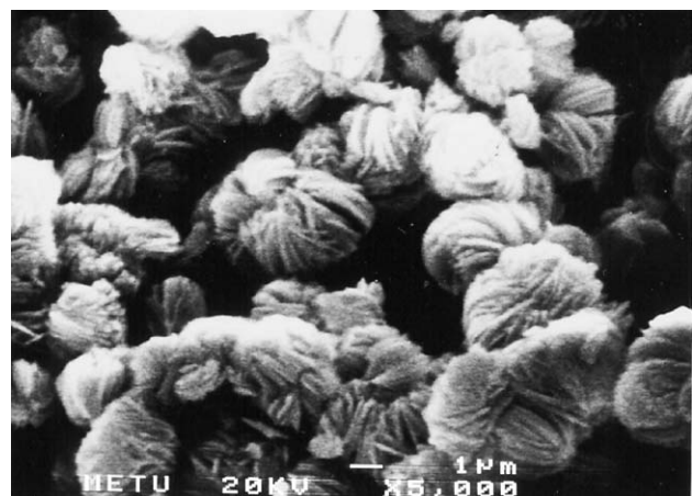
Fig. 5. Crystallized products having rosette morphology.
