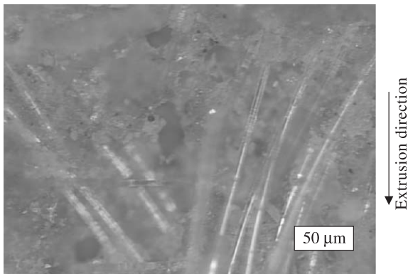
Fig. 5. The fiber distribution with 2% fiber volume ratio ( \times 500 ).
