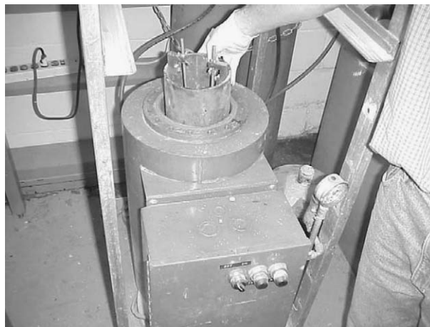
Fig. 2. Placing the metal container containing concrete specimen in the pressure chamber.
