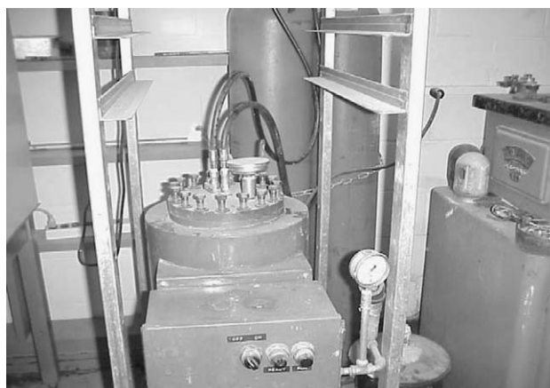
Fig. 5. Applying nitrogen pressure for epoxy penetration.
