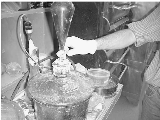
Fig. 4. Allowing ink to immerse specimen.
