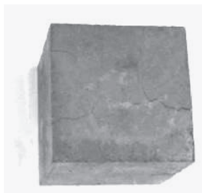
C-0.3-25 after exposure to 650°C
