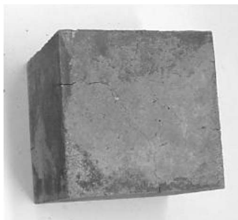
C-0.3-25 after exposure to 450°C (100mm cube)
