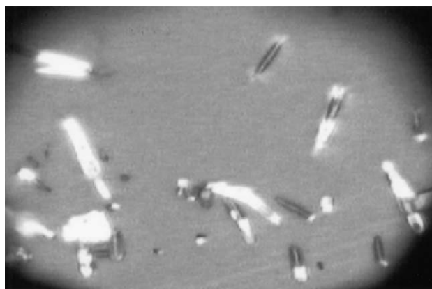
Micrograph 2. Aragonite needlelike crystal shape observed at \times 500 magnifications.
