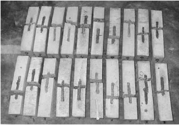
Fig. 4. Specimens after direct tension test.
