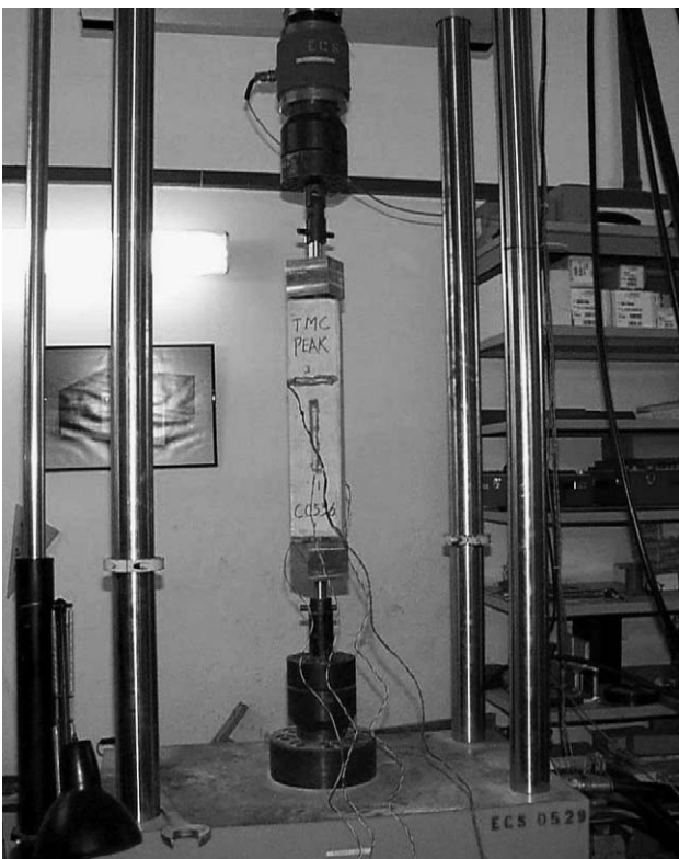
Fig. 2. Direct tension test using Instron testing machine.
