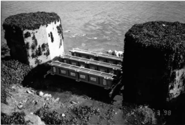
Fig. 12. Marine exposure site: concrete specimens at low-water-mark position.
