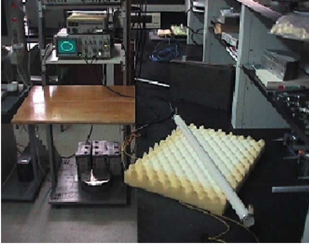
Fig. 1. Experimental setup used to validate the theoretical modeling. A cylindrical bar of concrete is mechanically excited by acoustic transducers. The transmission down the bar is detected by a second transducer. The voltage from both transducers is combined to form Lissajous figures on the oscilloscope screen.
