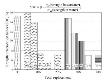
Fig. 8. Strength deteriorate factor at 10%, 20%, 30% and 40% cement replacements for 18 months curing.
