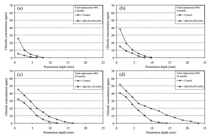
Fig. 5. Chloride concentration ingress profile with depth for 2, 4, 10 and 18 months at 40% cement replacement.
