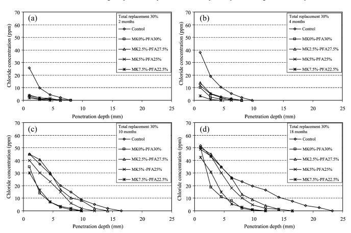
Fig. 4. Chloride concentration ingress profile with depth for 2, 4, 10 and 18 months at 30% cement replacement.
