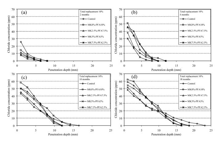
Fig. 2. Chloride concentration ingress profile with depth for 2, 4, 10 and 18 months at 10% cement replacement.
