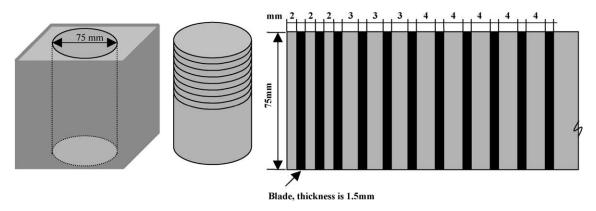
Fig. 1. Sample slices for chloride ingress profile measurement.
