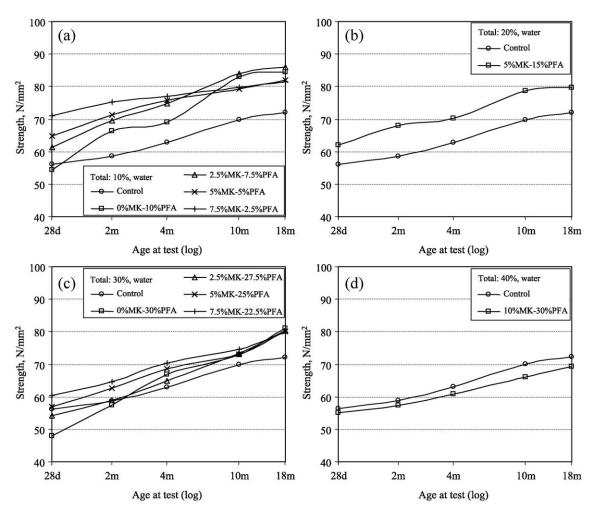
Fig. 6. Compressive strength with age at 10%, 20%, 30% and 40% cement replacements for water-cured concrete.
