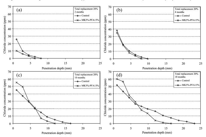
Fig. 3. Chloride concentration ingress profile with depth for 2, 4, 10 and 18 months at 20% cement replacement.
