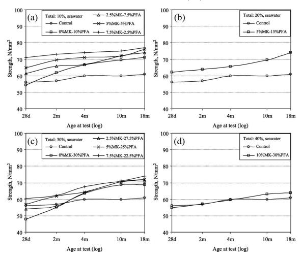
Fig. 7. Compressive strength with age at 10%, 20%, 30% and 40% cement replacements for seawater-cured concrete.
