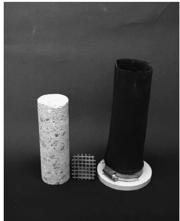
Fig. 3. Specimen in a rubber container, fully immersed into distilled water [8].
