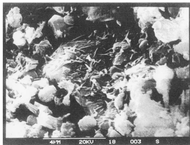
Fig. 10. SEM of the mixture without superplasticizer.
