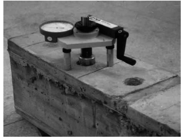
Fig. 2. Specimen for pull-off strength tests.
