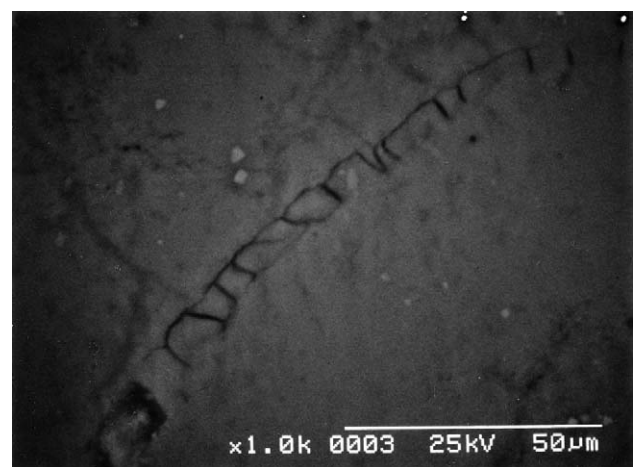
Fig. 7. BSE micrograph for the massive gels in 98-day-old mortar with 0.5% LiOH.
