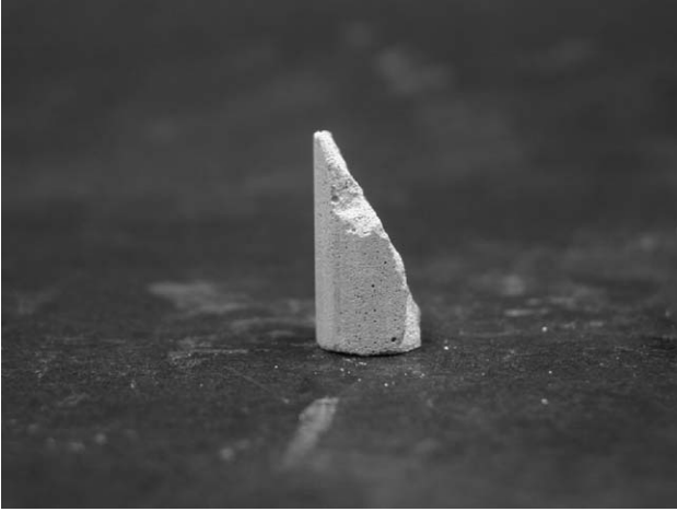
Fig. 13. Typical leached cement-paste specimen fragment after failure on the shear plane.
