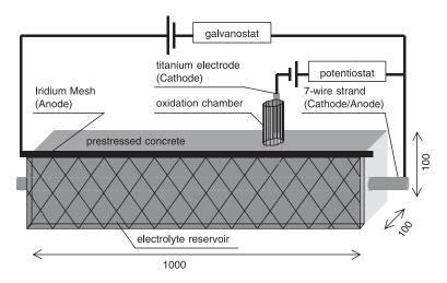
Fig. 2. Experimental set-up of prestressed concrete with a seven-wire strand.
