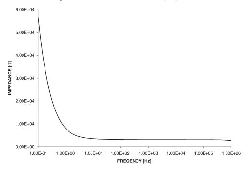
Fig. 10. Results of impedance measurement of calcium hydroxide solution through a 0.02-µm membrane.
