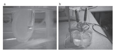
Fig. 3. Membrane in Perspex barrier (a) and experimental set-up (b).
