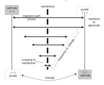
Fig. 1. Migration path of ions through membrane during impedance spectroscope measurements.
