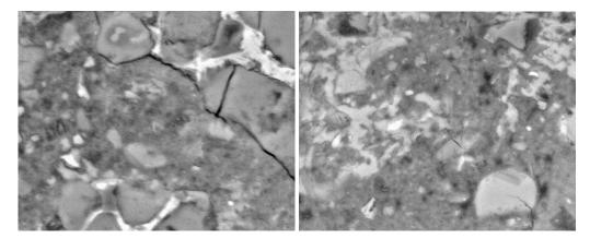
Fig. 9. SEM images taken from ECE-treated concrete at a distance of 42 mm from the reinforcement impression (Surface 4 Area 1 with 350 pores at  $0.46 \pm 0.06$   $\mu$ m and Area 3 with 265 pores at  $0.50 \pm 0.06$   $\mu$ m, average  $\pm$  S.D.).
