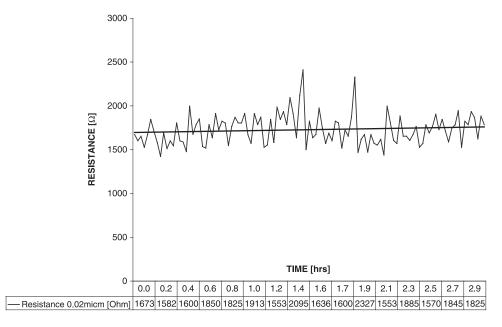
Fig. 11. Resistance of a 0.02- $\mu m$  membrane under DC regime.
