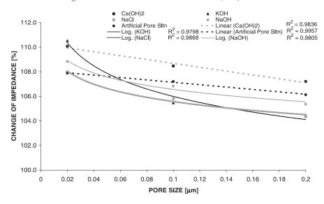
Fig. 12. Influence of pore size on impedance using different solutions (Table 5).
