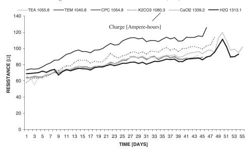
Fig. 4. Resistance of concrete samples with different electrolytes during ECE.
