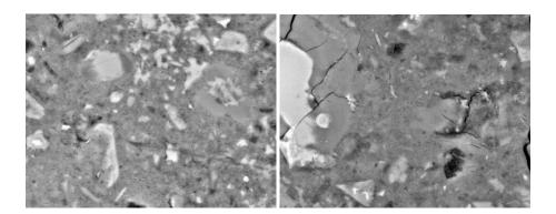
Fig. 7. SEM images taken from ECE-treated concrete at a distance of 16 mm from the reinforcement impression (Surface 2 Area 2 with 1011 pores at  $0.37 \pm 0.05~\mu m$  and Area 4 with 598 pores at  $0.41 \pm 0.06~\mu m$ , average  $\pm$  S.D.).
