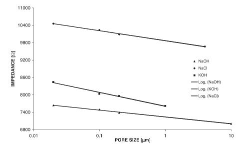
Fig. 14. Interpolated relationship between impedance range ( $10^6-10^{-1}$  Hz) and pore size of potassium and sodium hydroxide and sodium chloride solution; concentrations given in Table 5.
