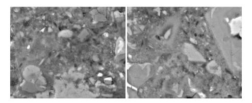
Fig. 8. SEM images taken from ECE-treated concrete at a distance of 29 mm from the reinforcement impression (Surface 3 Area 3 with 572 pores at  $0.37 \pm 0.05$   $\mu$ m and Area 4 with 497 pores at  $0.37 \pm 0.05$   $\mu$ m, average  $\pm$  S.D.).
