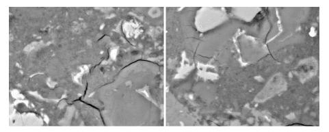
Fig. 6. SEM images taken from ECE-treated concrete at a distance of 3 mm from the reinforcement impression (Surface 1 Area 2 with 414 pores at  $0.33 \pm 0.05$   $\mu$ m and Area 5 with 443 pores at  $0.30 \pm 0.04$   $\mu$ m, average  $\pm$  S.D.).
