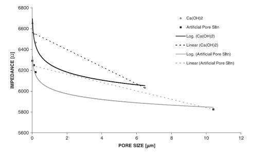
Fig. 13. Interpolated relationship between impedance range  $(10^6-10^{-1} \text{ Hz})$  and pore size of artificial pore solution and of calcium hydroxide solution  $[Ca(OH)_2]$ ; concentrations given in Table 5.
