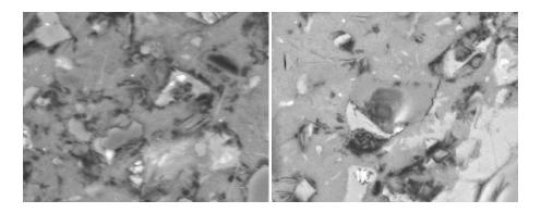
Fig. 5. SEM images taken from untreated concrete (Control Area 1 with 218 pores at  $0.85\pm0.09~\mu m$  and Area 3 with 169 pores at  $0.62\pm0.09~\mu m$ , average  $\pm$  S.D.).
