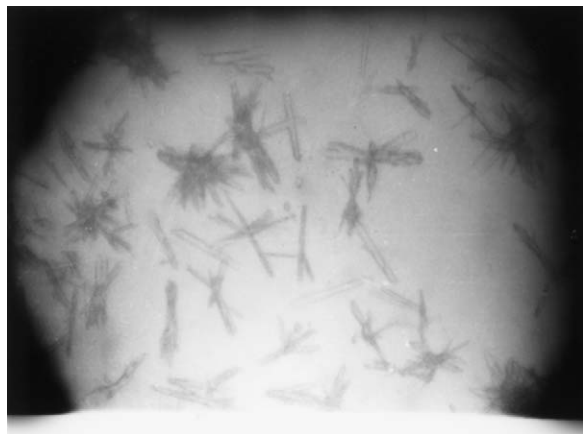
Fig. 6. Photomicrograph of hardened selenite plaster in the presence of 0.5% \text{CaF}_2 ( \times 45 ).
