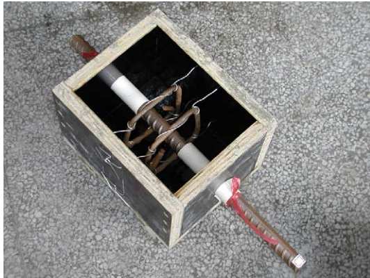
Fig. 3. Mould for specimens with stirrups.
