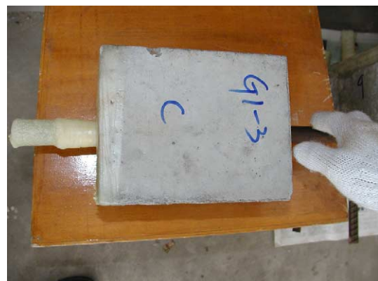
Fig. 5. Insulated end of steel bar during corrosion.
