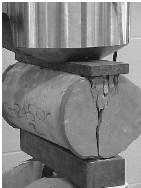
(b) Split tensile test
