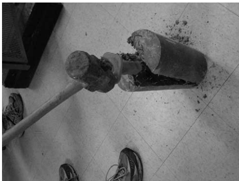
Fig. 5. Open a split tensile tested sample of rubberized concrete using a wedge and a hammer.
