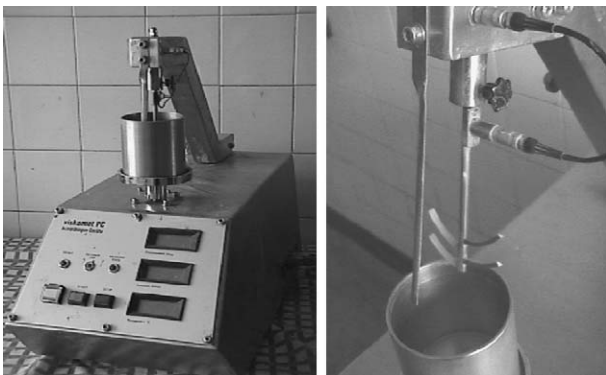
Fig. 1. Viskomat PC and its measuring element.
