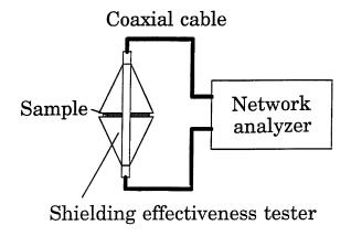
Fig. 1. EMI shielding effectiveness testing setup.
