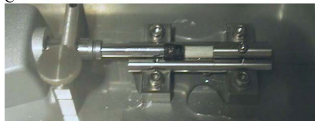
Fig. 2. (A) Experimental setup. (B) Three tablets (Ø4 × 9 mm) under length change measurement. (C) A prepared specimen (Ø4 × 10 mm) under measurement. (A–C) Water continually drops on the specimen to ensure a wet hydration environment in the specimens.
