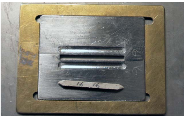
Fig. 4. Edge-shaped hardened specimen on top of the mould.
