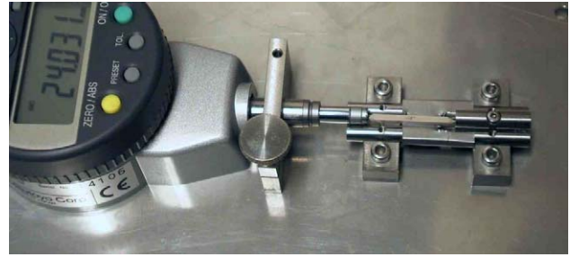
Fig. 5. The setup of the digimatic indicator.
