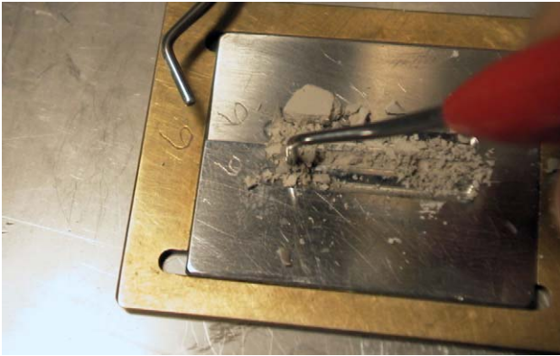
Fig. 3. Packing of pin specimens with dentist tools.
