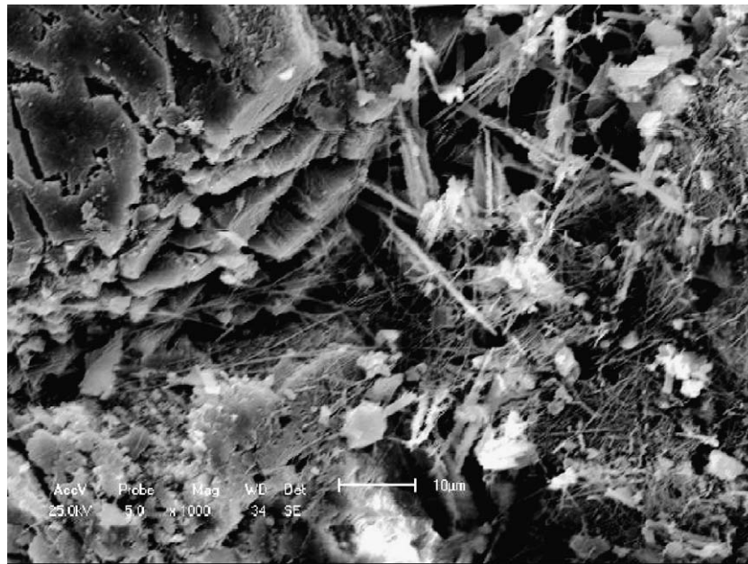
(a) Hardened cement paste, \times 1000
