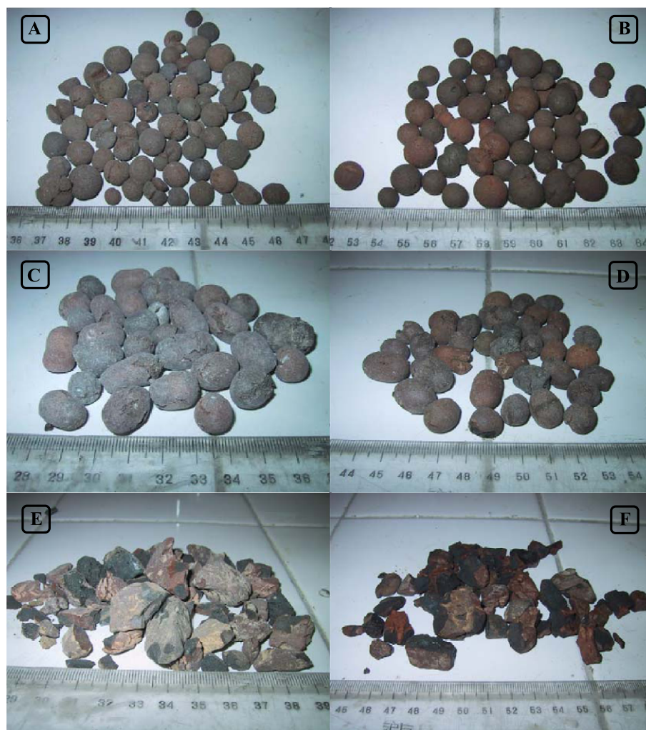
Fig. 1. Porous aggregates before and after absorbing PCM.
