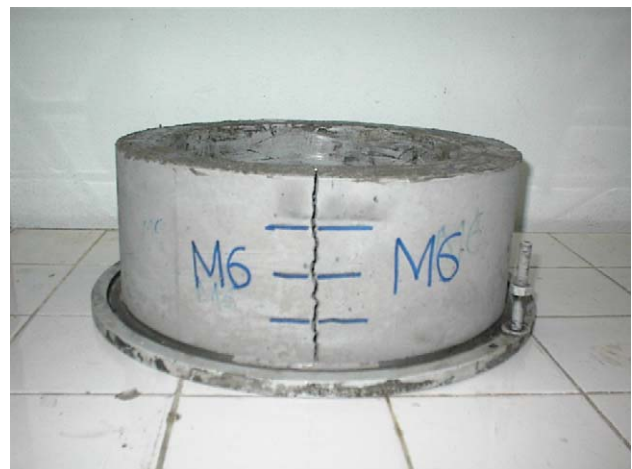
Fig. 2. Photographic view of a cracked ring specimen (M6).
