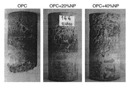
Fig. 1. Visual aspect of half buried specimens in sulfate soil for 10 years.
