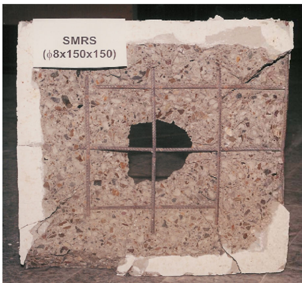
Fig. 6. Failure pattern of SMRS panel after the panel test.
