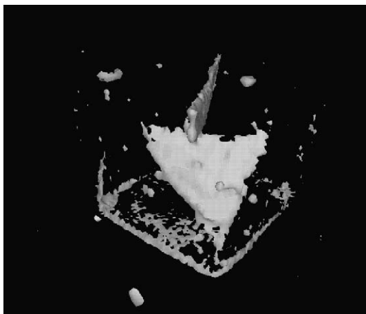
Fig. 10. Three-dimensional rendered spin-echo image of specimen A. The image orientation is similar to that of Fig. 4. The large synthetic crack is visible as well as the triangular crack of Fig. 6. The bottom of the image shows the rectangular structure of the specimen as a result of water condensing on the specimen surface. Droplet structures in the image are water condensed in the surface defects of the specimen.
