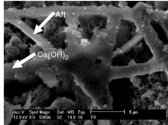
Fig. 3. Microstructure of normal concrete at curing age of 180 days.
