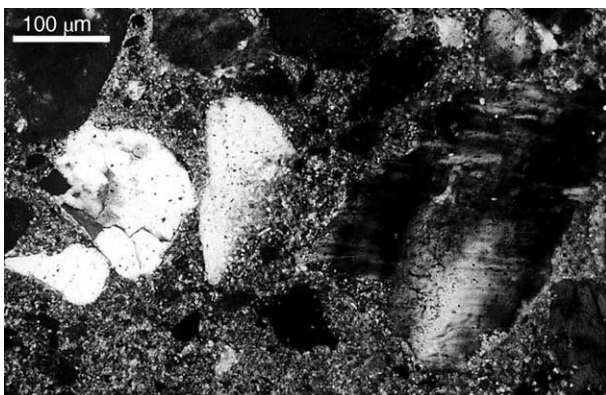
Fig. 5. Photomicrograph (crossed nicols) of a thin section of SNC mortar. Matrix dissolves the edges of skeletal grains (alkali–aggregate reaction).
