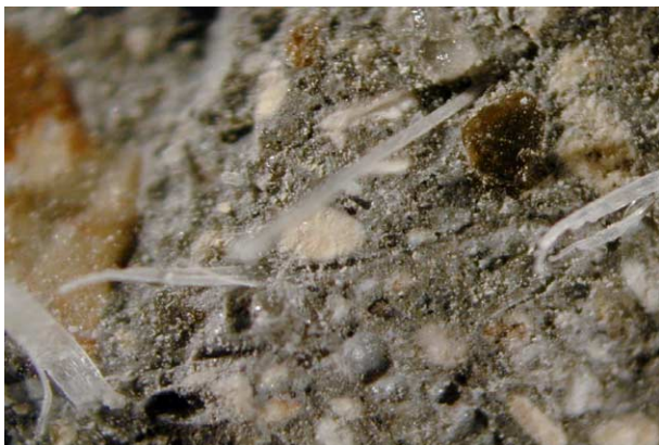
Fig. 3. Polypropylene fibres scattered in the high strength concrete.
