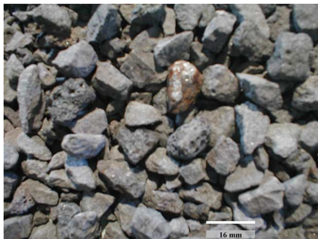
Fig. 1. A photograph of the ferrochromium slag used (the grain size in the range of 0–16 mm).
