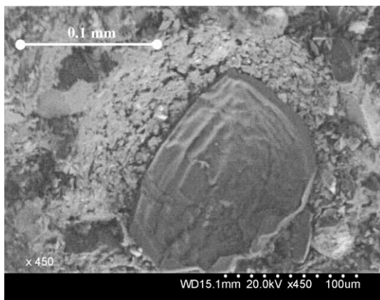
Fig. 4. SEM image showing paste backfill pore filled with secondary gypsum.
