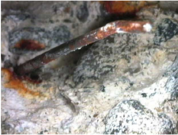
Fig. 12. Photograph of the corroded fibre in the crack.
